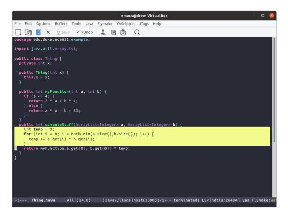
Now hit "C-c C-e" (the e is for extract method). Emacs will prompt you for the name of the extracted method (the default is "extracted"—lets change that to "dotProduct", then hit enter).
