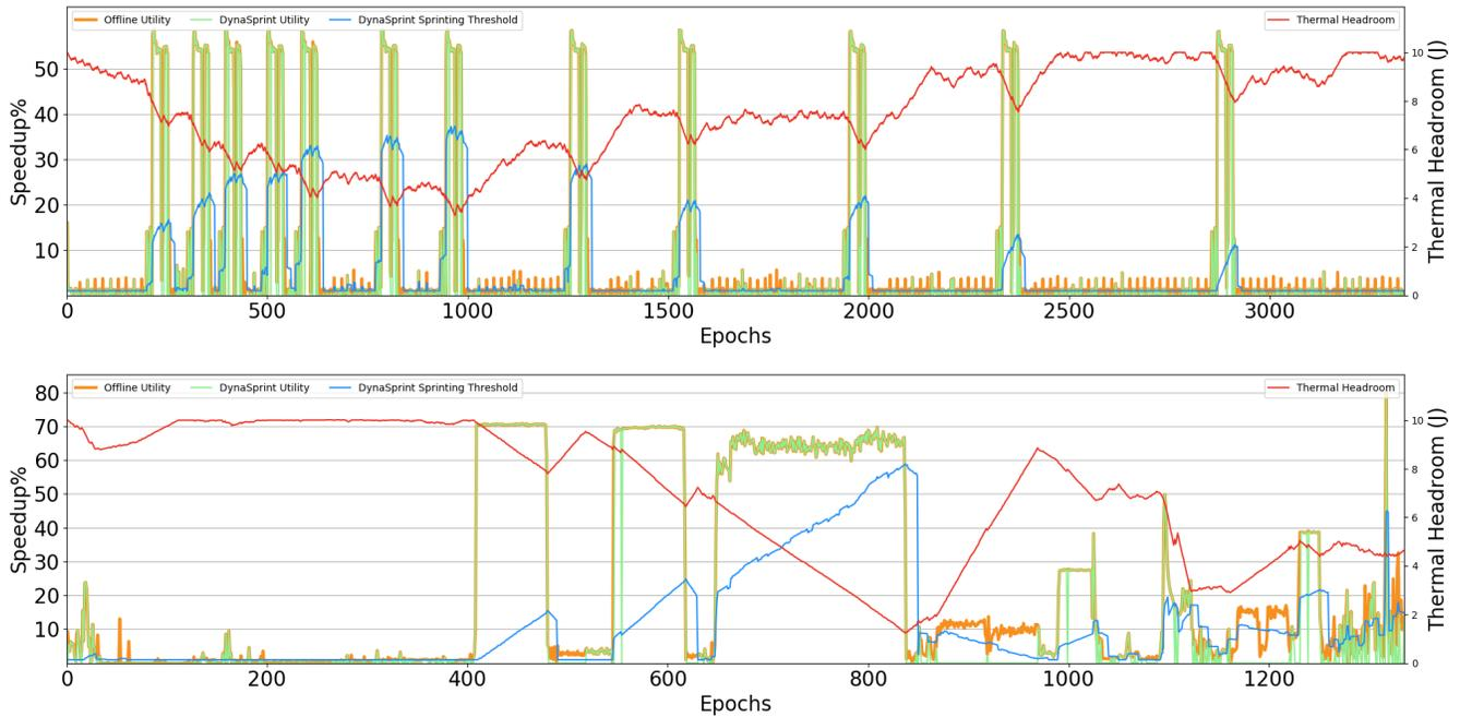
Figure 9: DynaSprint Sprinting Behavior: (a) ocean\_ncp, (b) gcc-s04
