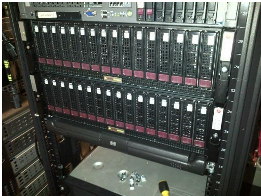
Two disk shelves and a storage server in a rack
